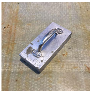
5 | Quick cooling. Cut away surplus filler with a chisel or cutting tool.
